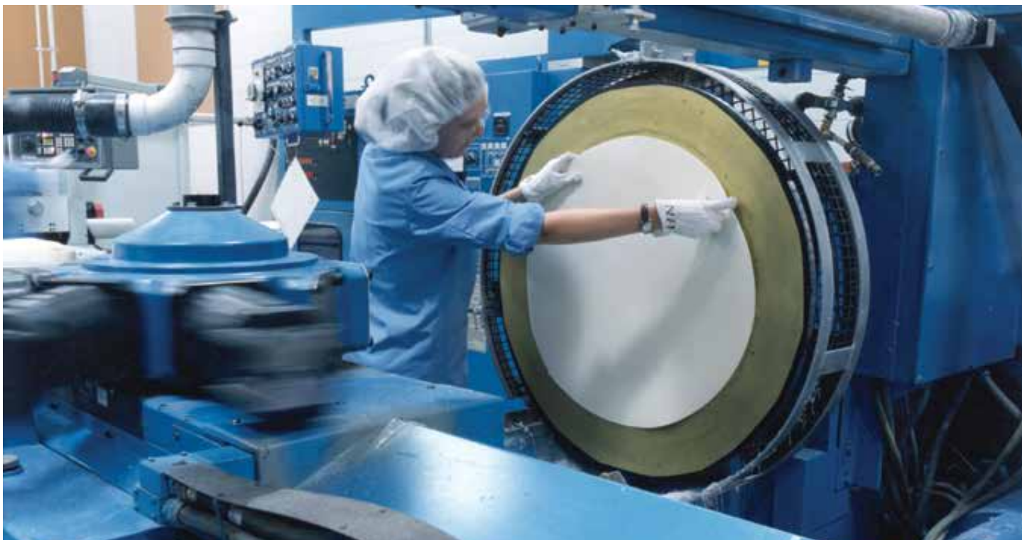
A Chemical Mechanical Planarization (CMP) operator is loading a polishing pad on a lathe for grooving. Dow CMP Technologies (CMPT) pioneered many of the pad products and processes that are widely used today and for over 30 years has remained the industry leader. CMPT offers a full range of polishing pads and slurries designed to meet the unique performance needs of each CMP application and node.
