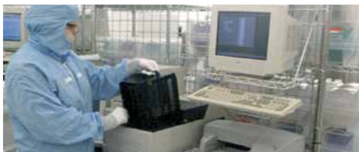
The Newark site has polishing labs that are designed similar to their customer's clean rooms where they make wafers containing chips. CMP technicians work in these clean room environments to develop and test new pad and slurry products that will be used by customers to make computer chips.
