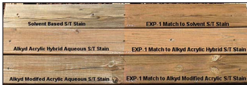
Figure 6—Thirty-month exterior durability of EXP-1 and commercial stains. After 30 months exposure at horizontal up, the EXP-1 stain has better durability (less flaking, erosion, and color fade) than the commercial semitransparent stains.
