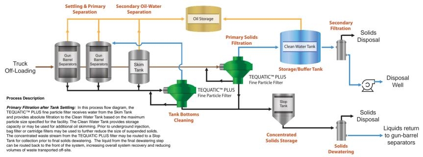
Tank Bottoms Cleaning: To further increase system efficiency, the debris that settles at the bottom of the Gun Barrel Tank and Skim Tank can be sent directly through the TEQUATIC PLUS filter, reducing the frequency of manual tank cleanouts. The clean filtrate would be sent back into the same tank and the concentrated waste stream would be routed to the Slop Tank for further dewatering. This process reduces the operating and maintenance costs, and downtime associated with tank bottoms cleaning.
